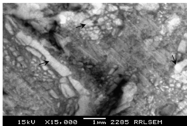
Fig. 4. SEM micrographs of the in situ Al–4Mg–AlN composite after 4 h reaction (gas flow rate: 0.4 lpm).
